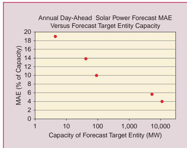
**figure 7.** The relationship of the annual day-ahead solar power forecast MAE (% of capacity) over all daylight hours to the installed capacity of the forecast target entity for a broad spectrum of entities (individual facility, regional, or system-wide aggregate).
